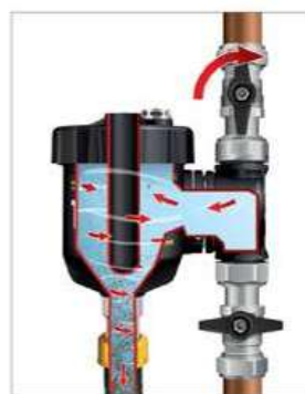
3. Open outlet and drain valves
